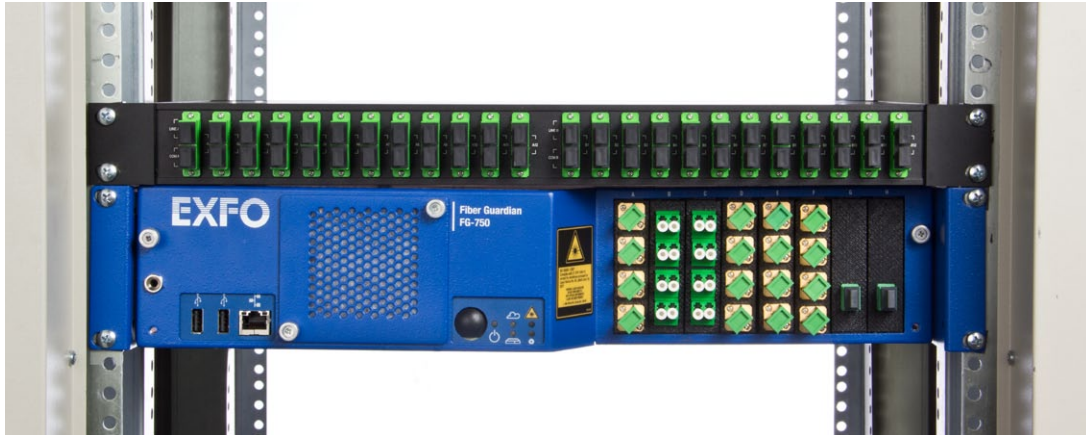
Figure 1. Typically sitting on top of or in the same rack as the Fiber Guardian unit, the TAM kit monitor ports are pigtailed at the rear (SC, LC, MTP -12f or MPO-8f) and connected to the front of the remote test unit.
