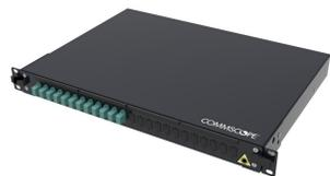
FMS Panel, 1U, 19 in, black, Includes 12 x LC OM4 Duplex Adaptors (24F), 24 x OM4 LC Pigtails. 24 x Splice protectors. Splice trays (2) and cable glands
