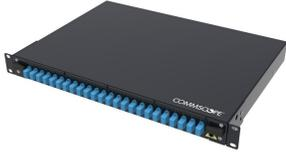
FMS Panel, 1U, 19 in, black, Includes 24 x LC SM Duplex Adaptors (48F), 48 x SM LC Pigtailed. 48 x Splice protectors. Splice trays (2) and cable glands
