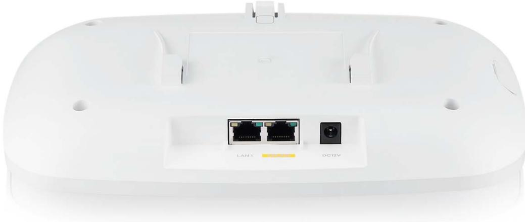
**Figure 32** WBE510D, NWA110BE Ports
