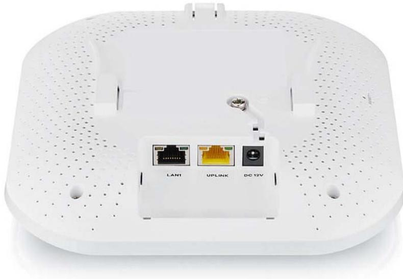
**Figure 27** NWA110AX, WAX510D Ports
