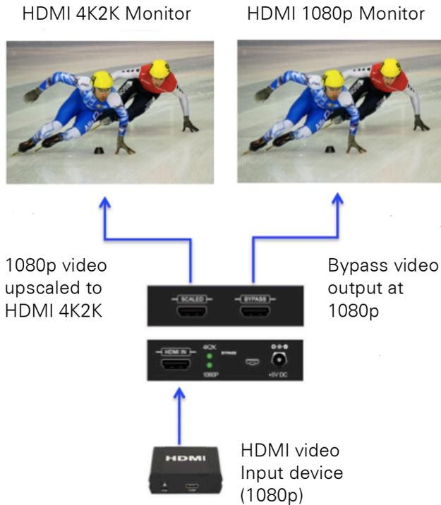
**Installation** This product is quick and easy to install. Power off all the video sources and monitors, then connect the HDMI cables from the HDMI 4K2K Scaler to the peripherals. Set the Bypass switch for video upscale or video downscale. Next, power on the HDMI Scaler, followed by the monitor and the video sources. When the input video signal is detected, the corresponding LED will illuminate.
