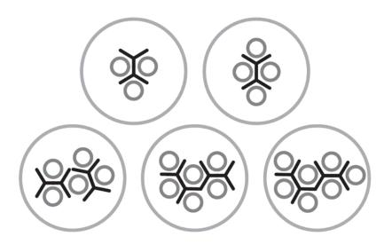
One TDUX clip seals up to 4 cables. If more cables are to be sealed, use one extra clip per 3 additional cables
