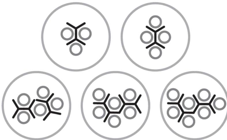
One TDUX clip seals up to 4 cables. If more cables are to be sealed, use one extra clip per 3 additional cables
