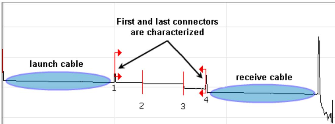
**Note:** To measure the loss in the first connector with the SPSB-EF launch cable, the OTDR pulse width should be 100 ns or shorter and the connection to the OTDR port should have a reflection value of -45 dB or better. A 50  $\mu\text{m}$  test link must also be selected.
