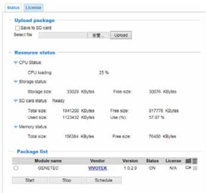
Users can store and execute VIVOTEK's or 3rd-party software modules onto the camera's flash memory or SD card. These software modules can apply in video analysis for intelligent video applications such as license plate recognition, object counting, or as an agent for edge recording, etc.
