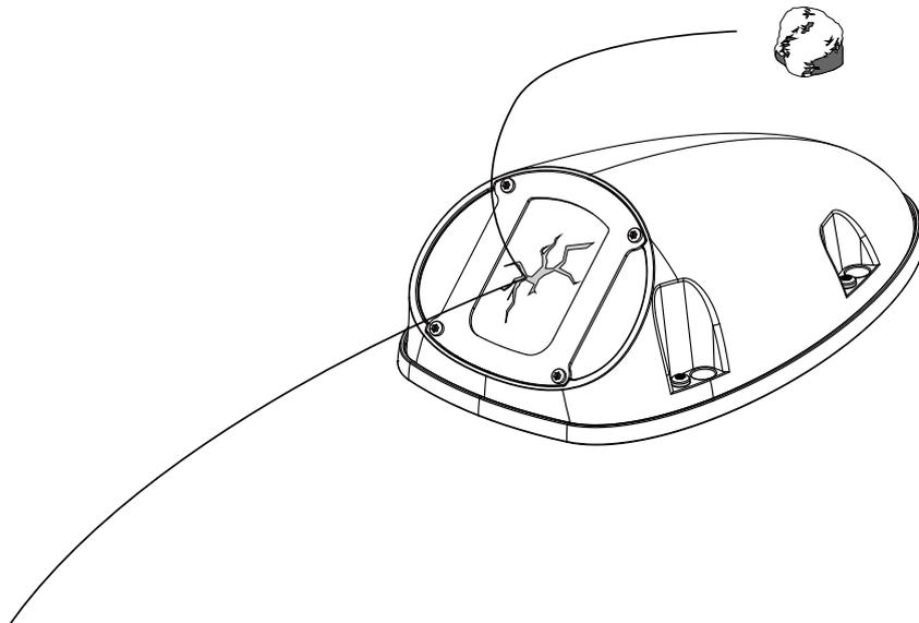
Remove the 4 T10 screws to remove the retention bracket. Replace the front window glass. Note that the heater pad should be placed at the original position.
