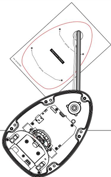
8. Secure the camera to the mount surface by driving 4 screws.
