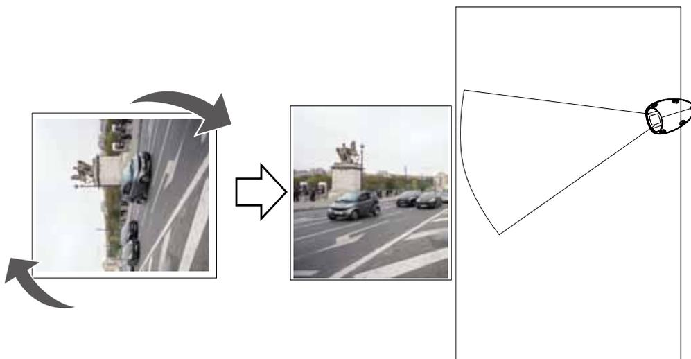
11. You can also use the twist adjustment ring to tune the image orientation if the need should arise.
