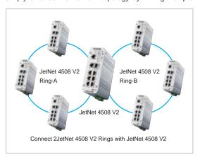
rings into a line or into multiple directions. In addition to extensibility, MultiRing TM has great diversity of various ring technologies. When MultiRing Menabled, JetNet 4508 V2 can connect RSR rings, TrunkRing Menabled a Super Ring together and simultaneously provide more Fast Ethernet Ring connectivities. This provides extensibility to new technologies while keeping the great backward compatibility.
