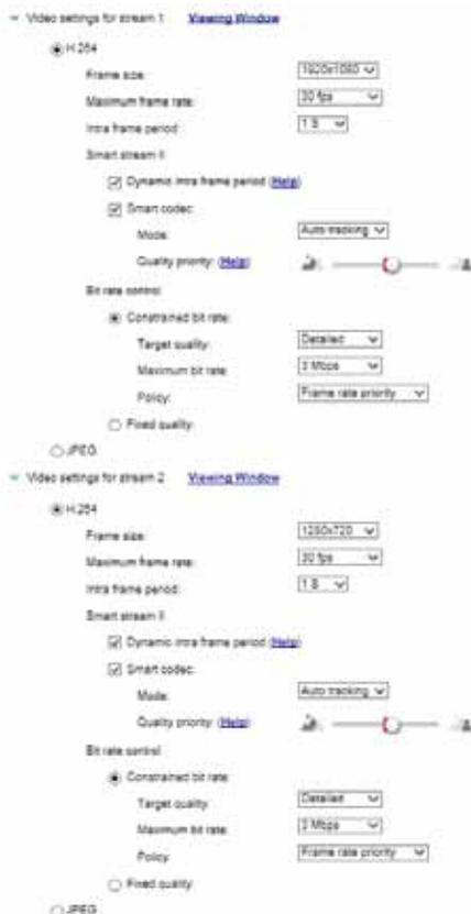
This Network Camera offers real-time H.264 and MJPEG compression standards (Dual Codec) for real-time viewing. If the **H.264** mode is selected, the video is streamed via RTSP protocol. There are several parameters through which you can adjust the video performance:
