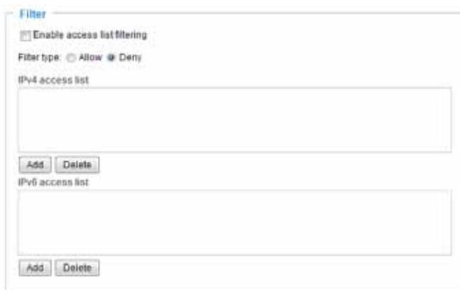
The screenshot shows a web interface for configuring filters. At the top, there is a checkbox labeled "Enable access list filtering". Below it, the "Filter type" is set to "Deny" (indicated by a selected radio button). There are two sections for access lists: "IPv4 access list" and "IPv6 access list". Each section has a large empty text area for input and two buttons labeled "Add" and "Delete" below it.
