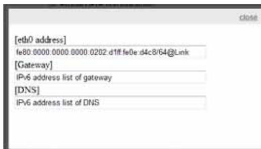
If your IPv6 settings are successful, the IPv6 address list will be listed in the pop-up window. The IPv6 address will be displayed as follows:
