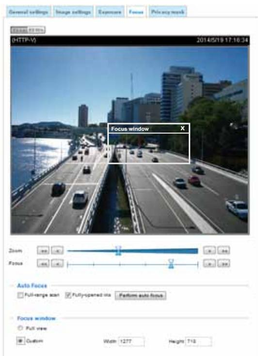
Below is the procedure to perform the automated Focus function:
