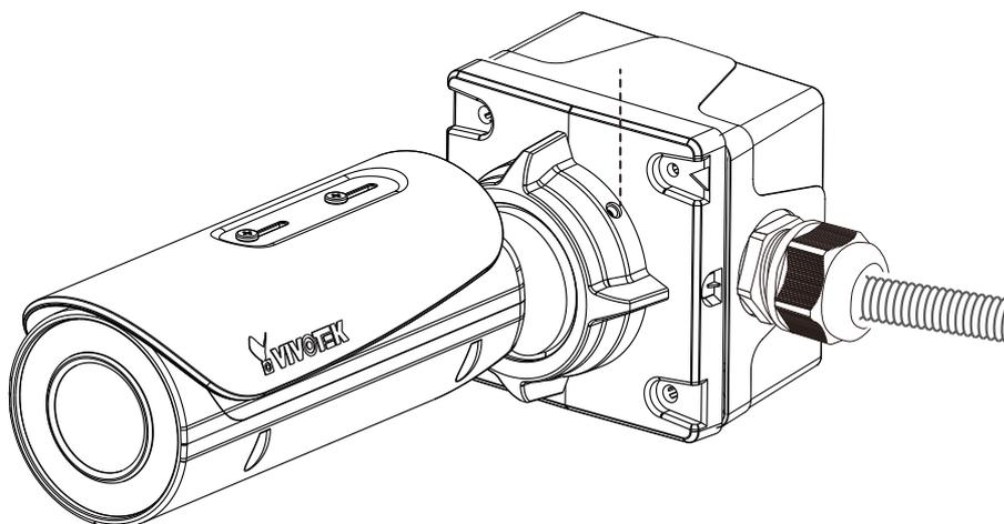
10. Loosen the fastening ring on the mount bracket using a hex wrench, and aim the camera at the area of your interest. When done, tighten the fastening ring.
