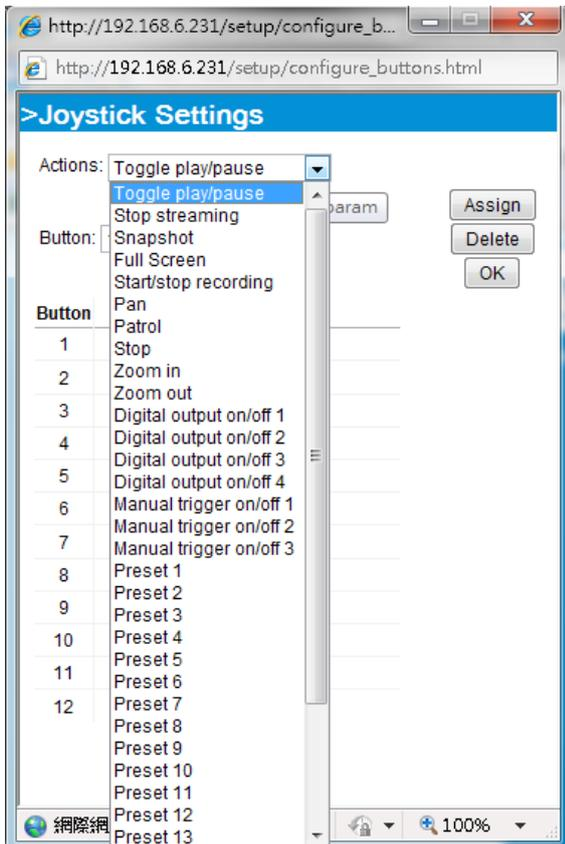
3. Click the **Assign** button to assign an action to the button. You can delete an association by selecting a button number, and then click the **Delete** button.
