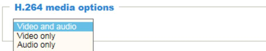
Select to stream video or audio data or both. This is enabled only when the video mode is set to H.264.
