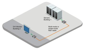
**Cables** Since the Transmitter and Receiver units have DVI male connectors, they connect directly to video sources and displays. They could also be connected with a short male-to-female DVI pigtail.
