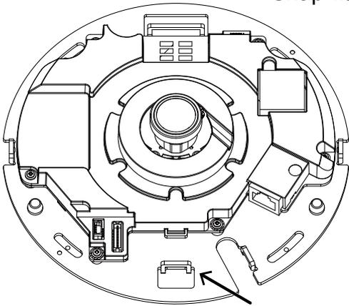
Install the plastic dome cover by aligning the snap-fit tabs on the dome cover with the slotted tabs on the camera base. Install the dome cover by pressing it evenly to the camera base.
