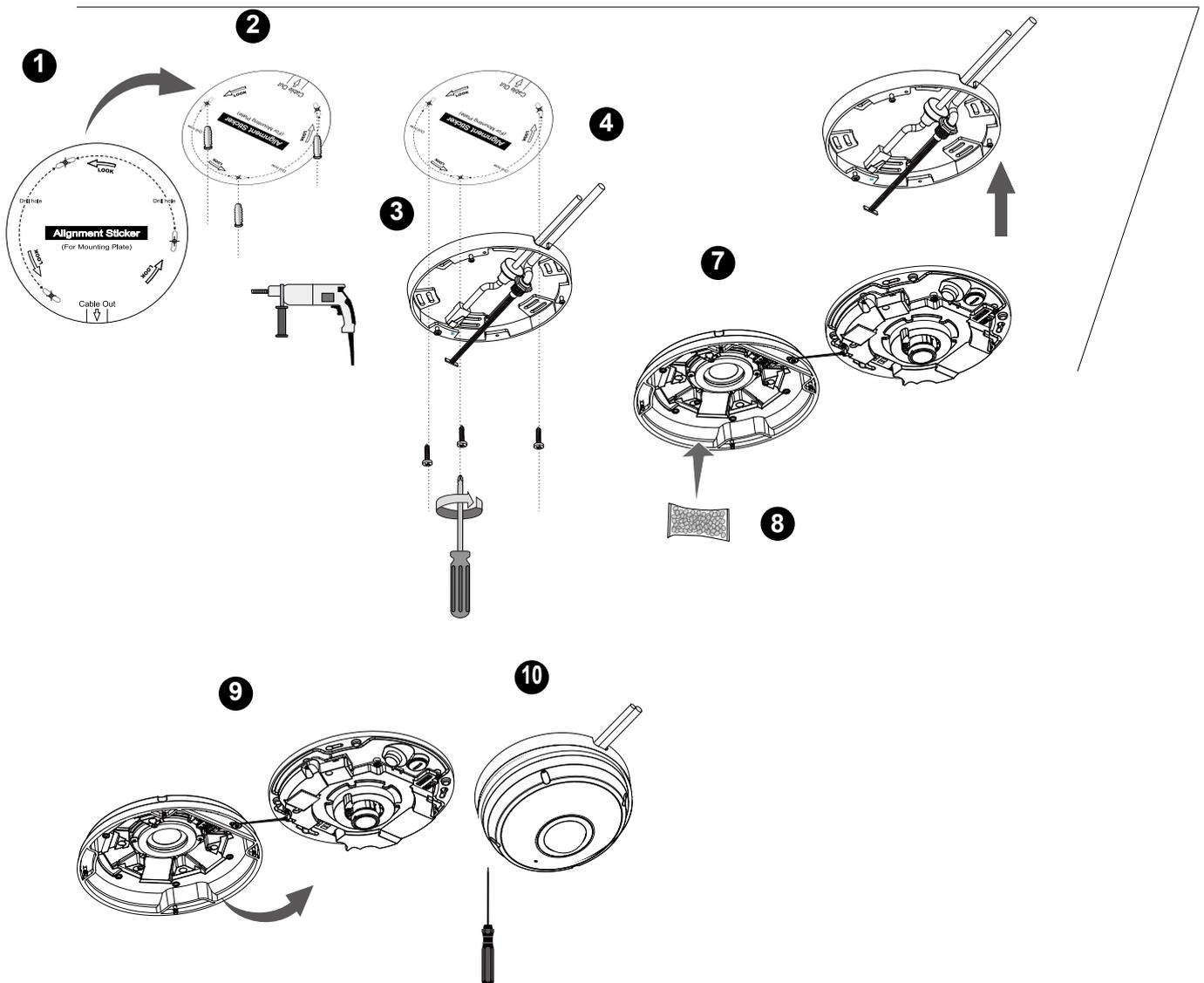
You may also use the diagonal holes on the mounting plate, marked as A, B, or C, to install the camera to a standard 4 in. junction box.
