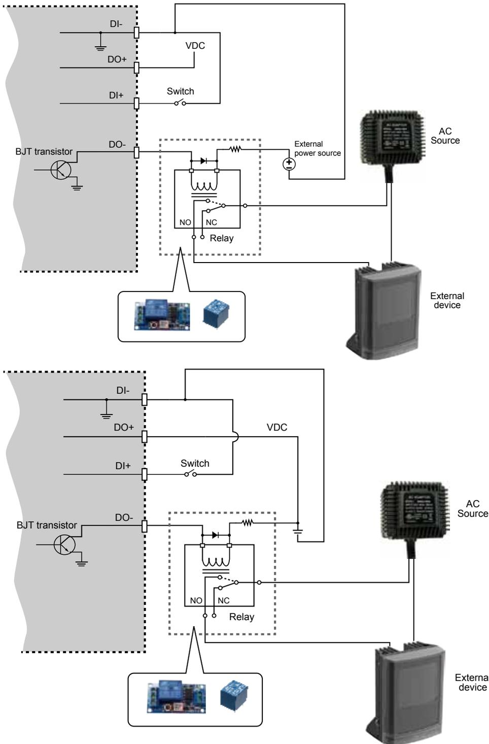
1. The DO+ pin provides 3.3V output, and the max. load is 50mA.
