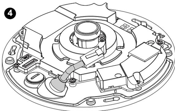
4. Feed the Ethernet cable from the bottom of the camera and through the hole. Attach the rubber seal plug for water proofing.
