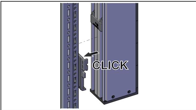
Fig. 12: Attach the PDU to the universal supports
