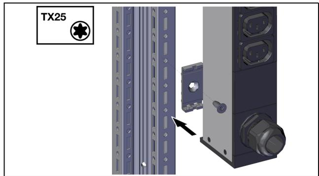
Fig. 10: Attach the PDU to the TS 8 rack
