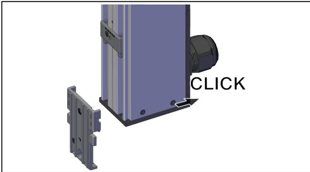
Fig. 7: Attach the universal support to the PDU
