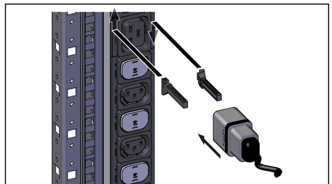
Fig. 14: Insert the brackets of the cable attachment
