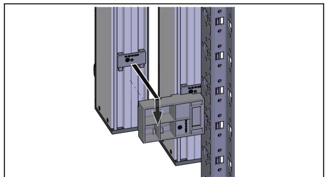
Fig. 6: Fit the second PDU in the extension
