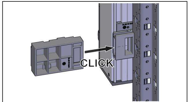
Fig. 5: Fit the extension to the TS IT bracket
