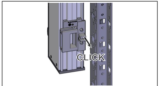
Fig. 4: Attach the PDU to the TS IT rack
