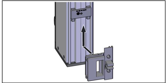
Fig. 3: Attach the TS IT bracket to the PDU
