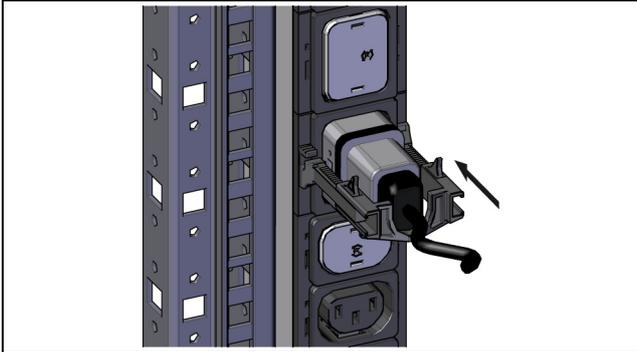
Fig. 15: Slide the cable attachment into place
