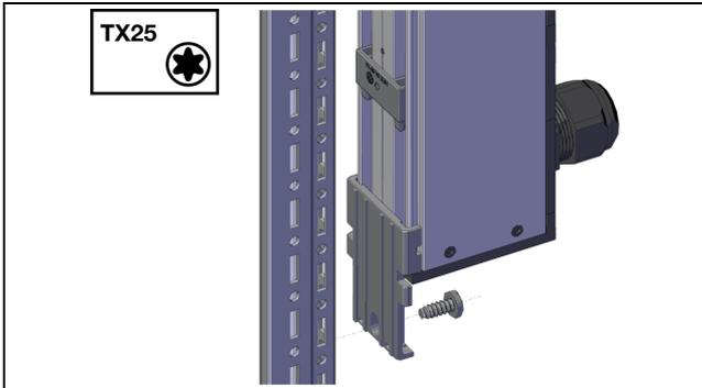
Fig. 8: Attach the PDU to the TS 8 rack
