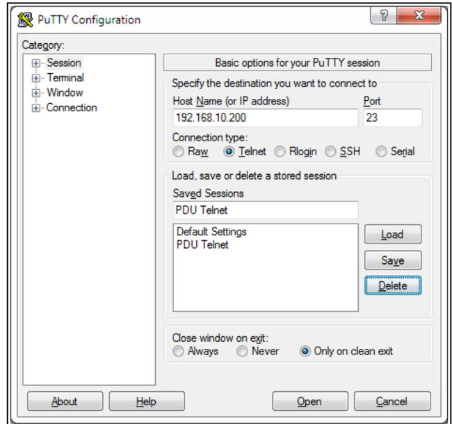
Fig. 23: Connection setting "PDU Telnet"
