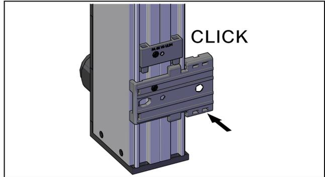
Fig. 9: Attach the universal support to the PDU
