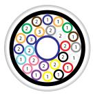
Microducts and outer sheath: HDPE Intermediate sheath: HDPE or PP
