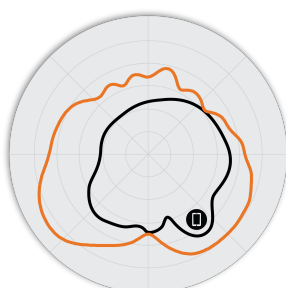
Figure 3. R350 5GHz Azimuth Antenna Patterns
