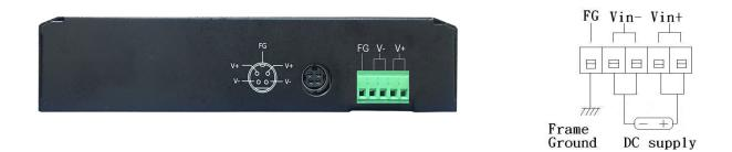
The DIN-4P connector on the rear panel also used for power input, you can use an AC/DC adapter with DIN-4P connector directly, recommends adaptor products is MS-180-56(56VDC/3.21A).
