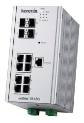
The JetNet 7612G-4F is an pure Gigabit industrial Ethernet Switch with 8 ports RJ-45, 4 ports Gigabit SFP socket for optical fiber network connection. It adopts high efficiency Ethernet MAC controller with 24Gbps Switch fabric bandwidth, 9K jumbo frame forwarding. The robust system design makes the JetNet 7612G-4F survive under harsh outdoor environment with extreme electric magnetic interference and the variation of environment temperature.
