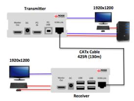
**Overview** The Xcion HDMI Extender is a robust and cost effective digital extension system, capable of being configured to suit most connectivity demands. Applications generally require digital video (1080p or 1920x1200) and USB-HID as standard. High-speed USB2.0 is available as an add-on option. Rack mounting options, a metal chassis and a DC power supply make this product particularly suitable for industrial extension environments.
