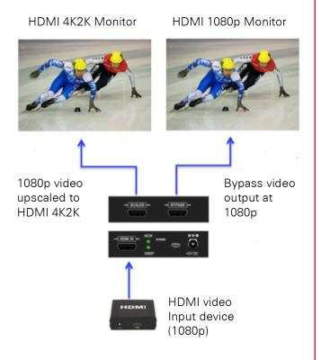
**Installation** This product is quick and easy to install. Power off all the video sources and monitors, then connect the HDMI cables from the HDMI 4K2K Scaler to the peripherals. Set the Bypass switch for video upscale or video downscale. Next, power on the HDMI Scaler, followed by the monitor and the video sources. When the input video signal is detected, the corresponding LED will illuminate.
