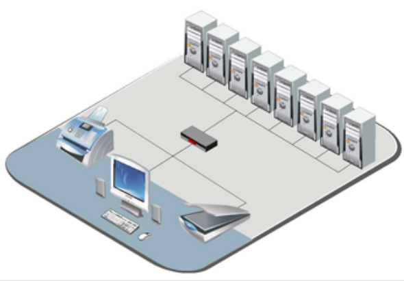
Vista CMH KVM switch with USB2.0 devices attached
