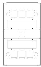
**Top Panel** 2off 130 x 448mm 6off 100 x 100mm 4off 60mm diameter DATA SHEET
