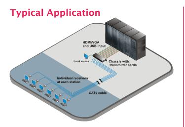
**Models** The CrystalView HDT is available in a single chassis model, which can host a combination of up to six HDMI or VGA Transmitter cards.
