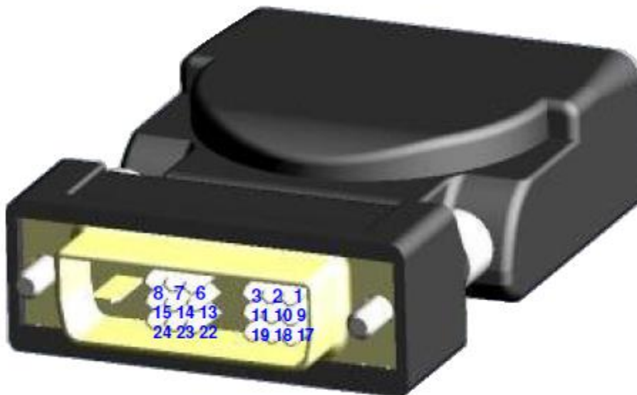
Figure 3 DVI-D Male (18+1) Connector PIN Definitions
