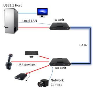
**Installation** Connect the transmitter to your computer or host device USB port. Connect the peripheral USB devices to the receiver unit. If there are more than four USB devices to connect, use a powered USB hub to expand the number of remote USB ports. Connect the transmitter to the receiver with up to 330ft (100m) of CAT6 cable. Use of CATx patch cables will significantly reduce the operating performance of the product. Apply power and the installation is complete.
