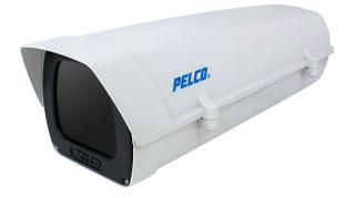
The **EH14 Series** enclosure offers two integrated power supply options for 24 VAC power input and 230 VAC power input; both units supply 24 VAC to the camera.
