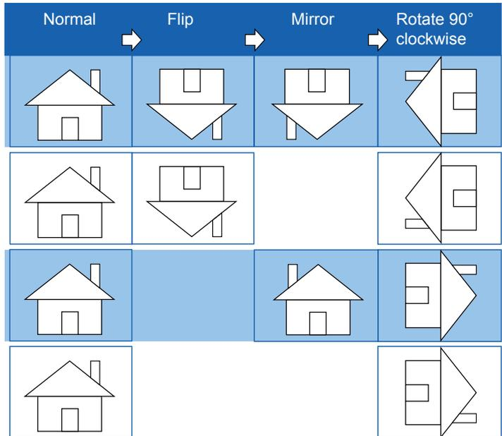
The camera may be installed on a vertical, side-facing, or tilted surface in order to accommodate the interior or exterior design of a vehicle or building. Because the interior of a transportation vehicle is often shaped as a narrow rectangular space, the conventional HD image, such as that of a 16:9 aspect ratio, will be incongruous with its wide horizontal view. With video rotation, the camera can more readily cover a tall and narrow field of view.
