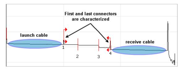
Note: To measure the loss in the first connector with the SPSB-EF launch cable, the OTDR pulse width should be 100 ns or shorter and the connection to the OTDR port should have a reflection value of -45 dB or better. A 50 µm test link must also be selected.
