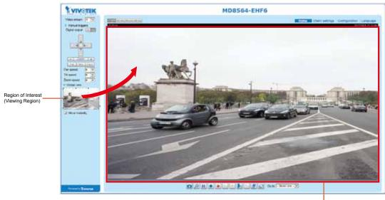
Output Frame Size (Size of the Live View Window) Click the stream item to display the detailed information. The maximum frame size will follow your settings in the above Viewing Window sections.
