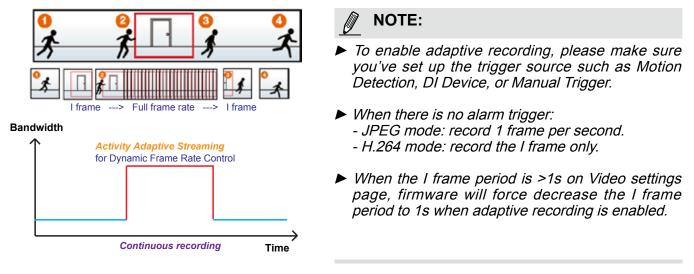
The alarm trigger includes: motion detection and DI detection. Please refer to Event Settings on page 109.
