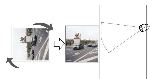
11. You can also use the twist adjustment ring to tune the image orientation if the need should arise.
