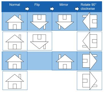
The camera may be installed on a vertical, side-facing, or tilted surface in order to accommodate the interior or exterior design of a building or vehicle. The interior of a building can be shaped as a narrow rectangular space, such as a corridor. The conventional HD image, such as that of a 16:9 aspect ratio, will be incongruous with its wide horizontal view. With video rotation, the camera can more readily cover the field of view on a tall and narrow scene.
