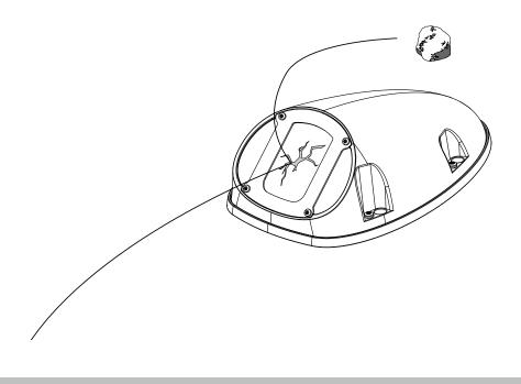
Remove the 4 T10 screws to remove the retention bracket. Replace the front window glass. Note that the heater pad should be placed at the original position.
