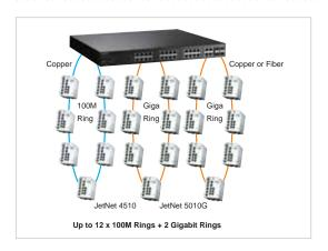
The JetNet 5728G-24P series supports the new generation ring technology – MSR<sup>TM</sup> which includes various new technologies for redundancy applications and structures of different networks. The PoE switch allows to aggregate up to 14 Rapid Super Rings, including 12 Fast Ethernet plus 2 gigabit Ethernet Rings. With the MSR<sup>TM</sup> technology, a node can be configured to multiple rings with the failover time in as little as 10ms, and zero-second of restoration time.
